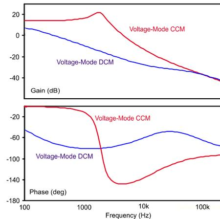
Fig. 4: Voltage-Mode Control in CCM and DCM
