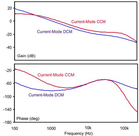
Fig. 5: Current-Mode Control in CCM and DCM
