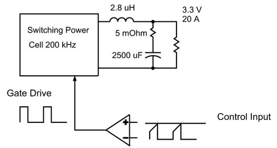
Fig. 2: Point-of-Load Buck Converter with Current-Mode Control
