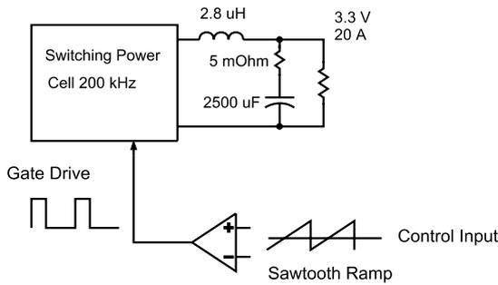
Fig. 1: Point-of-Load Buck Converter with Voltage-Mode Control
